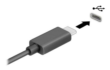
Connect the other end of the cable to the external device.
